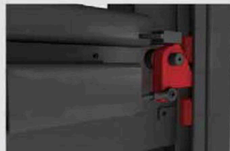
Mechanical anti-falling lock device to protect machine all the way
